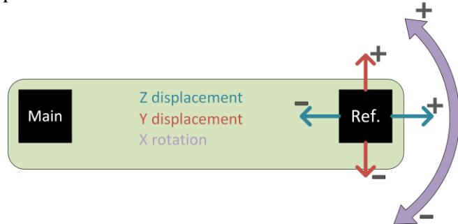
**Fig. 4.20.** Possible cases of magnetometer misalignment
