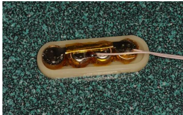
**Fig. 3.13.** Custom 3.1 V, 64 mAh battery pack
