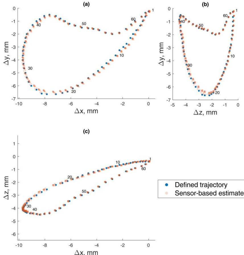
**Fig. 4.28.** The 5-DOF masticatory test trajectory estimated with BMF compensation and angle compensation; magnetic values at each point recorded with the sensor in the static state, mean localization error, and standard deviation
