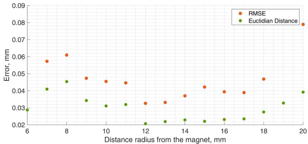
**Fig. 4.25.** Two-magnetometer localization approach with BMF compensation results from the FEM data; RMSE and average ED to the real sensor trajectory at different radii from the magnet
