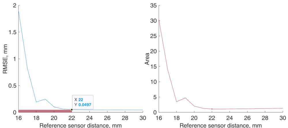
**Fig. 4.15.** (a) Dependency between localization RMSE and reference sensor distance to the main sensor, FEM data, (b) curve created by multiplying the localization error with corresponding magnetometer distance with the lowest point marked
