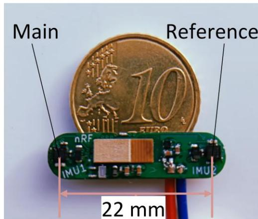
**Fig. 3.12.** The prototype of the wireless two-magnetometer sensor
