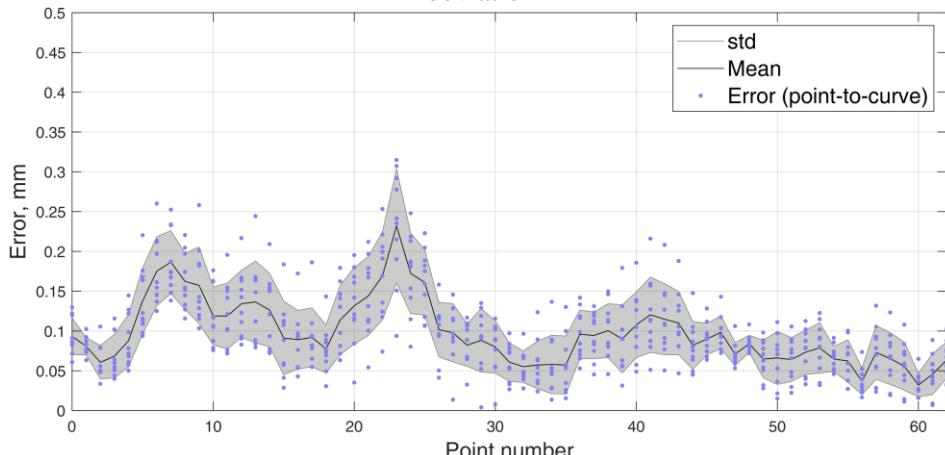
**Fig. 4.30.** Static 5-DOF experiment; localization (point-to-curve) ED error for every point measurement during 10 trajectory iterations with the mean and standard deviation
