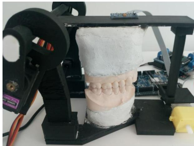
**Fig. 3.4.** Single-hinge vertical motion articulator with attached IMU
