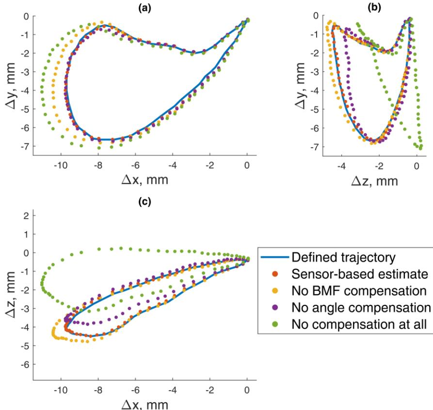
**Fig. 4.36.** The 5-DOF masticatory test trajectory estimated with and without the BMF compensation and jaw angle estimation algorithms; magnetic field values at each point recorded with a sensor in the static state: (a) lateral–vertical view (x–y), (b) protrusive–vertical view (z–y), (c) lateral–protrusive view (x–z)
