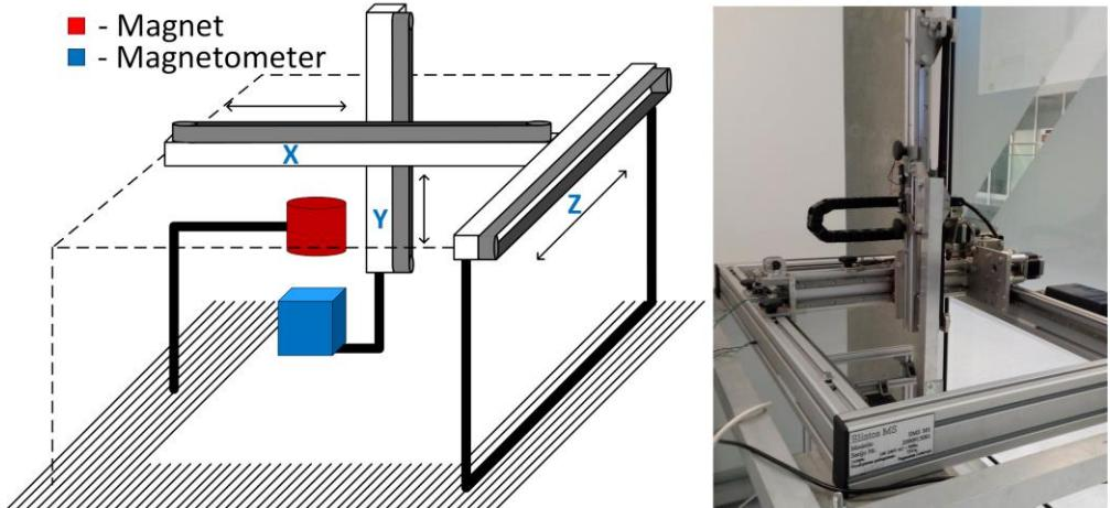
**Fig. 3.3.** Experimental setup (left) and 3D positioning system “EMS 301” (right)
