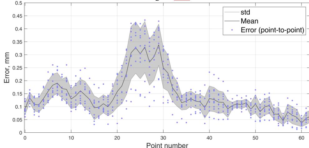
**Fig. 4.29.** Static 5-DOF experiment; localization (point-to-point) error RMSE of every point measurement in 10 trajectory iterations with the mean and standard deviation
