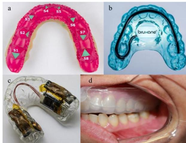
**Fig. 1.5.** Splints for bruxism diagnostics: (a) attrition-based splints for semi-automatic inspection by 3D scanning [24], (b) Bruxane splint with integrated pressure sensors [25], (c) splint with integrated piezoresistive pressure sensors [5], (d) splint with optical fiber sensors [26]
