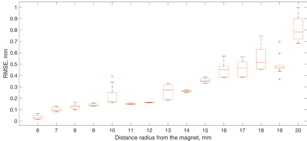
**Fig. 4.26.** 10 measurement RMSE median and standard deviation for the experimental measurements at different radiiuses from the magnet
