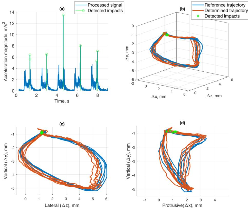
**Fig. 4.6.** (a) Teeth impacts detected by an experimentally selected threshold of  $5 \text{ m/s}^2$ , set on acceleration the vector magnitude value (RSS of X, Y, and Z components); (b) masticatory trajectory determined by the magnetic position tracking and reference methods while detected teeth impacts are marked at the points of detection, 3D view; (c) lateral–vertical view (z–y); (d) protrusive–vertical view (x–y)
