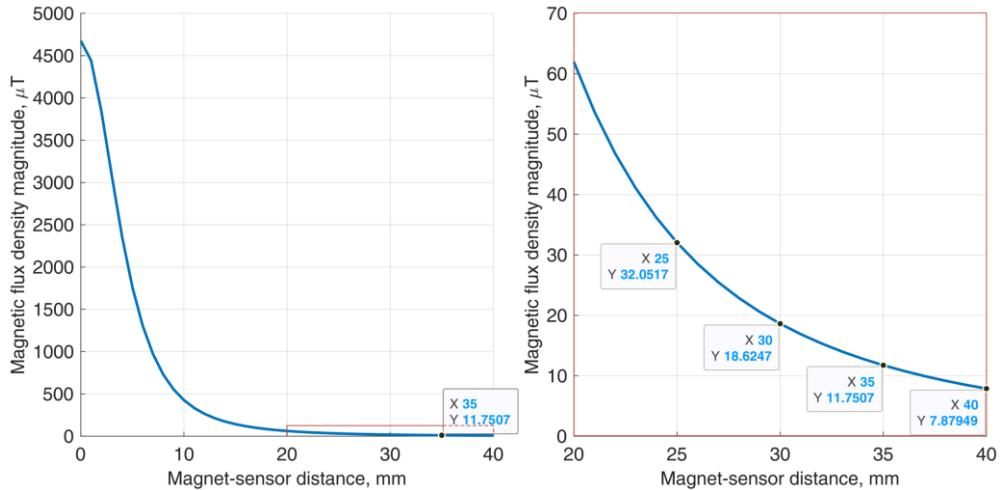
**Fig. 4.8.** Dependency of the magnetic flux density magnitude to the magnet-sensor lateral distance (x) at constant 6 mm vertical distance (y) (start of the dynamic range), marked area zoomed on the right
