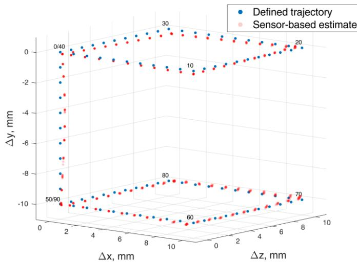
**Fig. 4.1.** Cubic test trajectory drawn with a 3D positioning system (blue) and determined from the magnetic field values (red); the numbers from 0 to 90 represent all measured points, while transparent markers show sensor-based estimate of 10 iterations of each point
