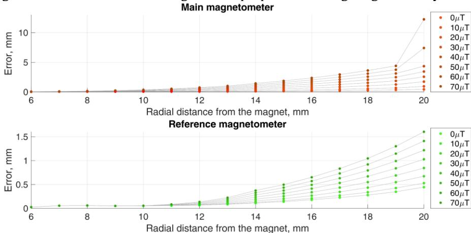
**Fig. 4.19.** The magnitude of error expressed in RMSE, caused by various main and reference magnetometer zero-offset changes at different magnet-to-sensor radiiuses throughout the proposed working range of the system
