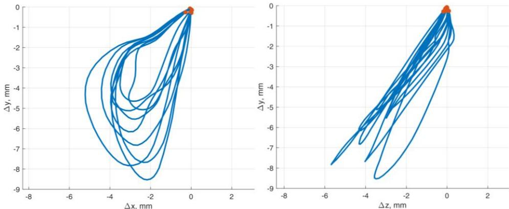
**Fig. 4.35.** Sensor-based estimate of a masticatory motion recorded intraorally with detected teeth impacts marked in red; front and side projections
