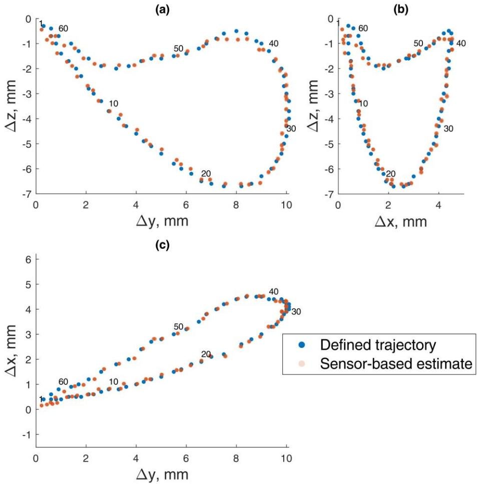
**Fig. 4.3.** Test masticatory trajectory drawn with a 3D positioning system (blue) and determined from the magnetic field values (red); the numbers from 0 to 62 represent all measured points while transparent markers show sensor-based estimate of 10 iterations of each point: (a) lateral–vertical view (y–z), (b) protrusive–vertical view (x–z), (c) lateral–protrusive view (y–x)
