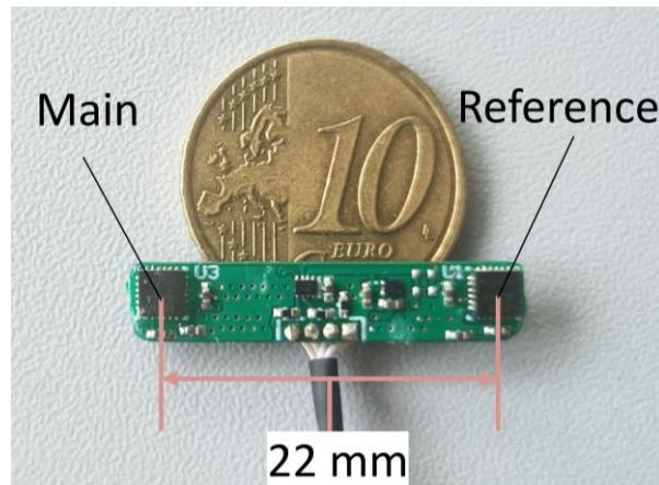
**Fig. 3.11.** Prototype sensor board with two magnetometers
