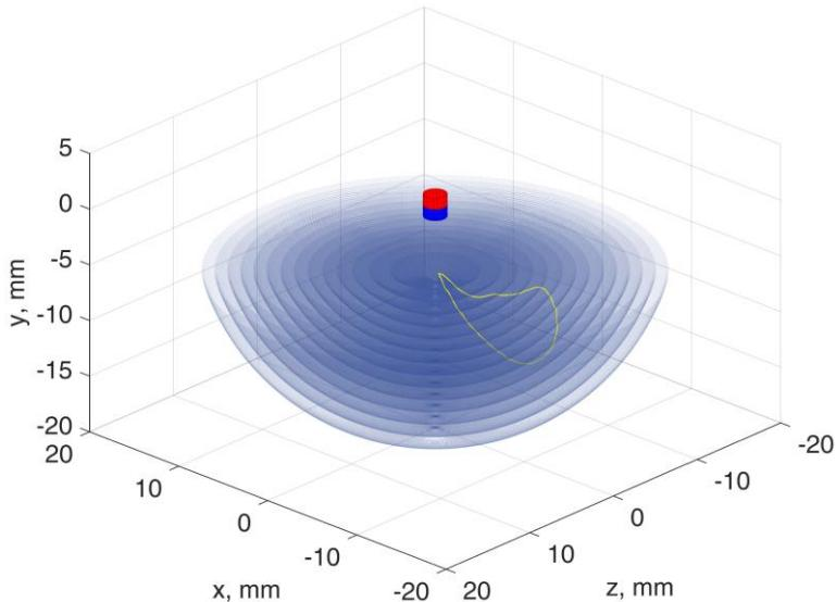
**Fig. 3.18.** Working range divided into spheres at different radiuses from the magnet, from 6 to 20 mm; 6 mm is the minimal magnet-to-sensor distance; the previously used test masticatory curve is included for scale
