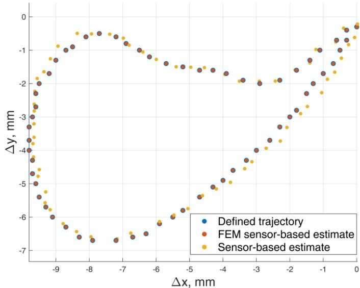
**Fig. 4.12.** Original input trajectory and estimated trajectory while using BMF compensation from FEM simulation data, RMSE = 0.05 mm (red), and the prototype sensor, based data with natural BMF, RMSE = 0.28 mm (yellow)
