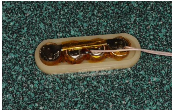
Fig. 3.13. Custom 3.1 V, 64 mAh battery pack
